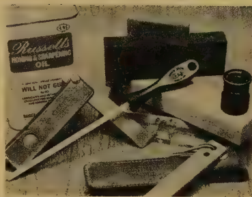
Accessories to aid in keeping an edge on your knife. Honing steels are by Gerber and Schrade-Walden. The long thin rod is a Moon Stick by Case, an excellent tool for quick touchup. The large white sharpening stone is a Washita/Soft Arkansas stone, and the large black one is the Surgical Black to be used as a final touch for razorlike sharpness. The loupe is for examining the blade edge. Russell's oil may be purchased quite inexpensively in large cans.
